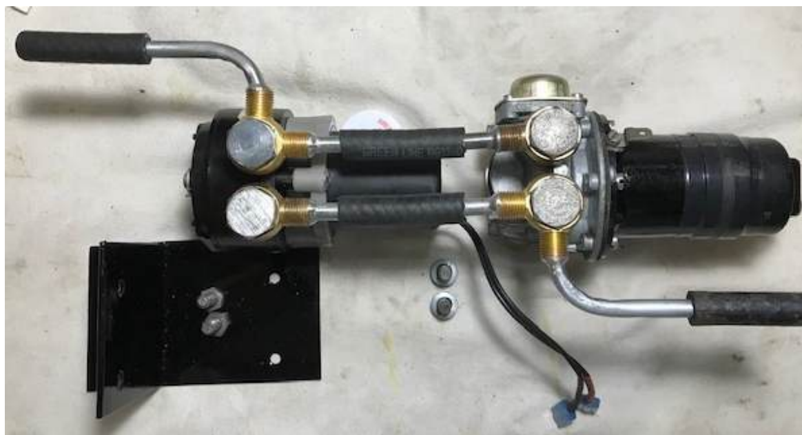
Photo #7: Dual pump mock-up on the workbench. Hose connections will be made using spring clamps. Lower left is the new pump bracket
