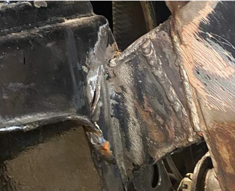
THE RESONATOR Rear crack cleaned up
